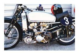
This rare machine was an AJS V2 ,water cooled Super Charged machine. It looks as though it may have been a handful on the track. But an interesting design.
