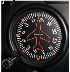
This Gyroscopic Compass can be set manually before flight and then monitored for compass alignment during flight, it can of
