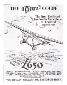
It is quite amazing that this aircraft was designed in 1926 as an enclosed two seat monoplane fitted with an Armstrong Siddeley five cylinder engine producing 110 HP.
