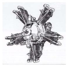
The cylinders can be seen protruding into the airstream for cooling efficiency.
