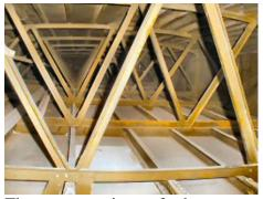
The construction of the centre section ribbing continued to the outer section and filled with fuel which gave the 2,500nm range.
