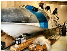
The fuselage is released from its large wing after 70 years and is being prepared for trestling, even so the minimum width of the hull is 10ft 6" when the wheels are retracted. The length remains at 61ft and height at 14ft or a bit less.
