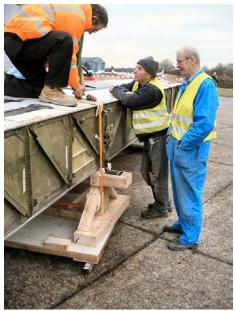
Attaching trestles, for lifting onto the second transporter.
