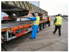
This centre section was 27 inches in depth and 8 feet wide. Basically a fuel tank, the outer wing sections tapered toward the wingtip were 30 feet in length. They too, were part of the fuel tank.
