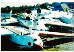
Good formation to the bitter end...! These aircraft were secured to the concrete by their wing points, which were no match for the strength of the hurricane.
