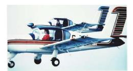
Air Touring was equipped with a Rallye aircraft the most used the 880B. To check fuel levels there was a glass tube on the cockpit side panel. Due to its non-stallable characteristic, it was soon known as the "metal parachute".
